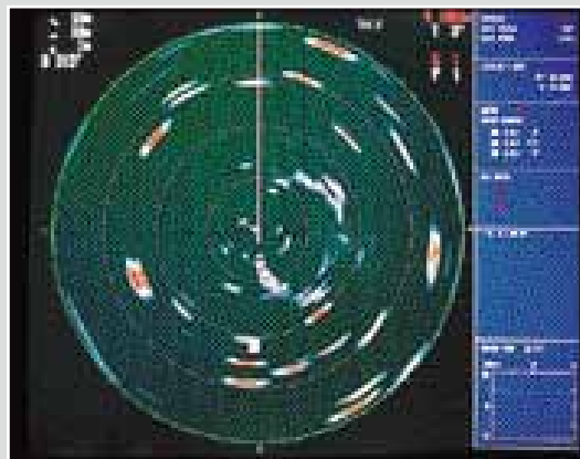
Full-circle display showing net formation in relation to the target fish schools
