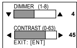
*Dialog box for adjustment of panel illumination, display contrast*
