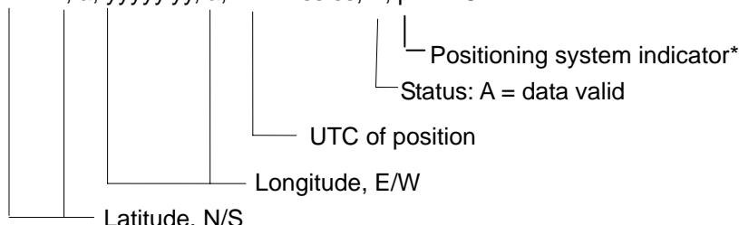
\*A = Autonomous, D = Differential, E = estimated(dead reckoning), M = Manual input, S = Simulator, N = Data not valid. The Mode indicator field supplements the Status field. The Status field shall be set to V=invalid for all values of Operating Mode except for A=Autonomous and D=Differential. The positioning system Mode indicator and Status field shall not be null fields.
