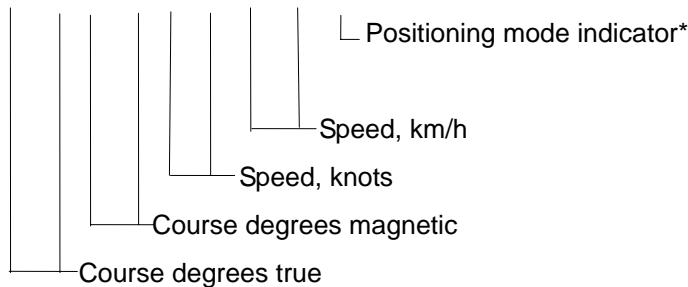
\*A = Autonomous, D = Differential, E = estimated(dead reckoning), M = Manual input, S = Simulator, N = Data not valid. The Mode indicator field supplements the Status field. The Status field shall be set to V=invalid for all values of Operating Mode except for A=Autonomous and D=Differential. The positioning system Mode indicator and Status field shall not be null fields.
