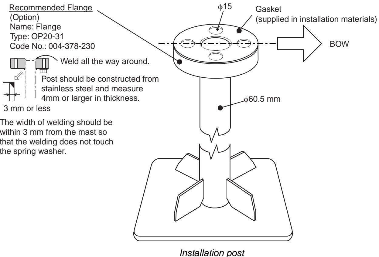
2. Fix the antenna unit to the post as shown below.
