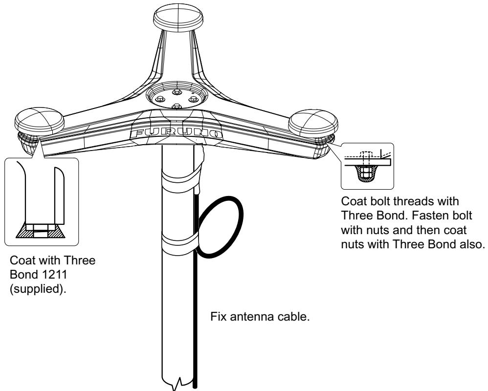
5. Coat bolt threads with Three Bond 1211.
