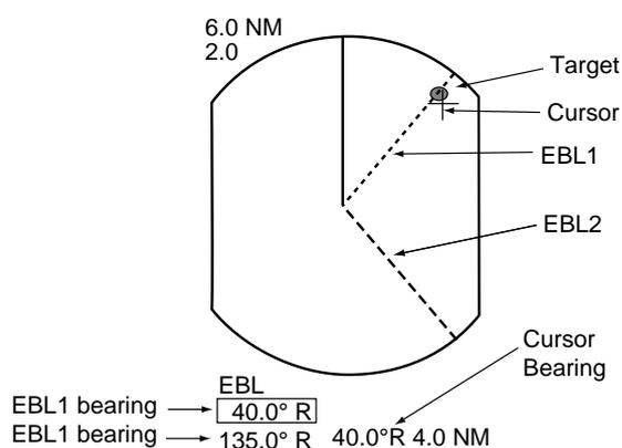
Figure 2-9 How to measure bearing by EBL and cursor
