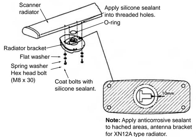
Figure 6-18 Fastening the radiator to the radiator bracket
