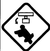
**Turn off the radar power switch before servicing the antenna unit. Post a warning sign near the switch indicating it should not be turned on while the antenna unit is being serviced.**
