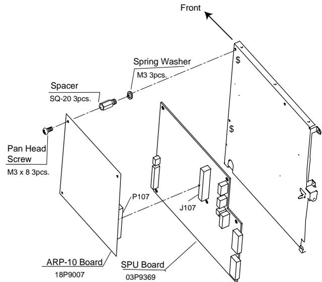
\$: Pull the front panel slightly to fix these screws.
