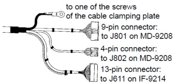
Figure 6-6 Signal cable, antenna unit side
