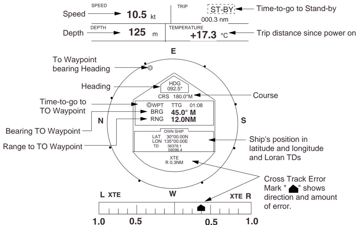
Figure 2-3 Typical navigation data display during stand-by
