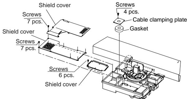
Figure 6-5 Antenna unit, inside view
