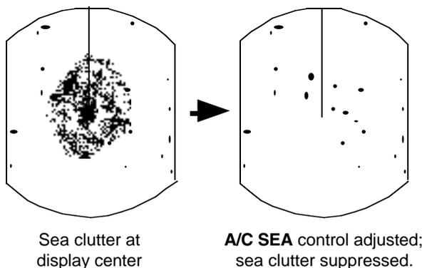
Figure 2-4 How to adjust the A/C SEA control
