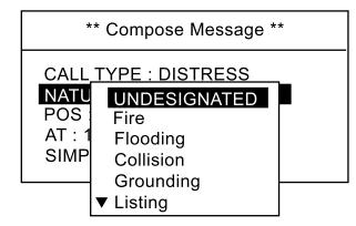
2. Rotate the channel knob to choose the nature of distress. On the remote handset, press the up or down arrow key.
