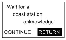
If you do not receive DIST ACK from coast station within five minutes and your vessel meets requirements (see previous page) for transmitting DIST ACK, select CONTINUE by the CHANNEL knob and press the ENT key. The following window appears.
