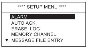
2. Rotate the **CH** knob (or press up / down arrow key) to choose MESSAGE FILE ENTRY and press the **ENT** key.
