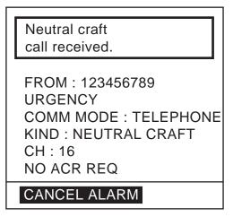
2. Press the **CANCEL** or **ENT** key. The audible alarm is silenced and the display changes as below.
