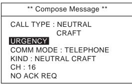
5. Press the **CALL** key more than three seconds to transmit the call. After the call is transmitted, the standby display appears with CH16 selected.
