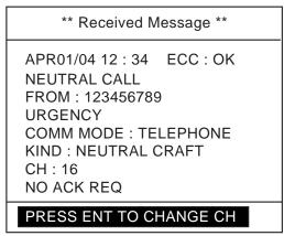
3. Press the **ENT** key. The display changes to the standby display, indicating CH16.
