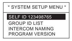
3. Rotate the **CH** knob (or press up / down arrow key) to choose INTERCOM NAMING and press the **ENT** key. The following window appears.
