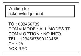
2. When the ACK from the coast station is received, the following display appears. The communication time (charge time) is informed.
