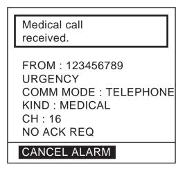
2. Press the **CANCEL** or **ENT** key. The audible alarm stops and the display changes as below.
