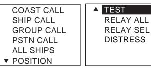
3. Rotate the **CH** knob (or press up / down arrow key) to choose DISTRESS. Press the **ENT** key.
