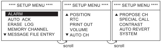
Rotate the CH knob (or press up / down arrow key) to choose SYSTEM from page 3 of the menu and press the ENT key. The following window appears. The self ID is displayed on the first line.
