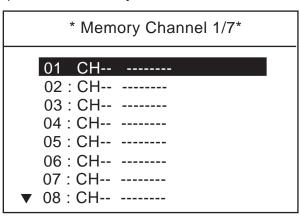
3. Rotate the **CH** knob (or press up / down arrow key) to choose a vacant CH number and press the **ENT** key.
